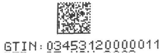
Figure 4-1 Inkjet printed GS1 DataMatrix
